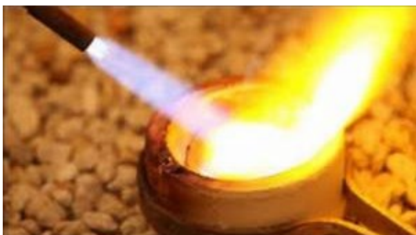
Gold mixed with flux (white powder) refined under intense heat
